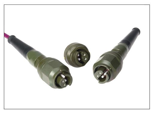
The Hermaphroditic Quad connector has been designed specifically to facilitate the interconnection of fibre optic cable assemblies, thus eliminating the need for polarising the assemblies and the use of inline adapters. The HQM series utilises ceramic sprung loaded ferrule technology, giving low repeatable optical attenuation.
