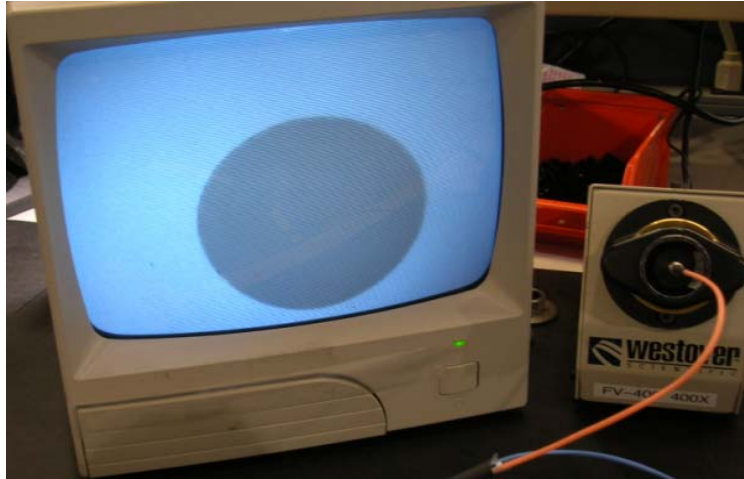
Figure 5 - Video Display of Ferrule and Fiber End Face
