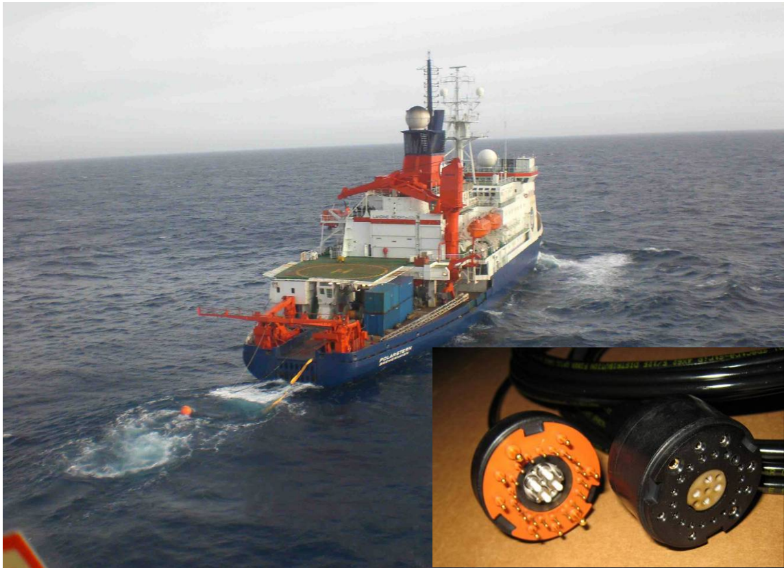
Figure 5. Oil exploration ship with hybrid streamer interconnect
