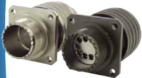
MIL-PRF-64266 style (NGCON) compliant fiber optic connectors are designed and manufactured using proven technology and features from existing connector standards of D38999 and M28876. These innovative connectors include genderless contacts and high-density packaging. This connector family includes innovations such as rear-release genderless contacts, wide temperature range and high-density packaging. AFSI also offers the companion M29504/18, /19 and /20 style termini for this connector suite.
