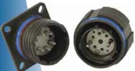
AFSI offers ARINC 801 cylindrical fiber optic connectors. Based on the commercial ARINC 801 specification, this series features a removable insert for termini end face cleaning, guide pins for precision alignment and a scoop proof shell design. It is available in standard D38999 plug and wall mount shells. Inserts are available to support 2 to 32 termini.
