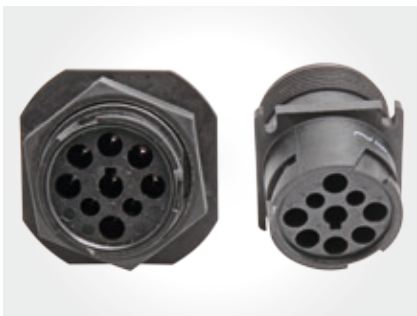
AT CIRCULAR (J1939) The AT Circular series is a moulded thermoplastic receptacle, the interface is in accordance with the J1939/13 diagnostic connector.
