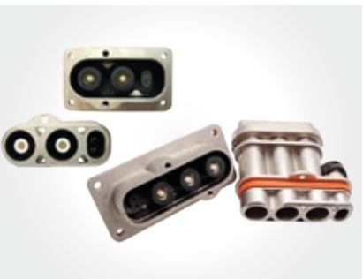
EPOWER The ePower series of connectors feature RADSOK® technology and are designed for the demanding requirements of hybrid, electric vehicles, and utility truck electrical systems, operating at 800 V DC to 1,000 V DC with a 200 A to 500 A rating.
