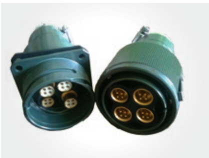
ASGTC-QUADRAX Circular bayonet lock connector for Data line transmission, IP67 protection, self-locking system
