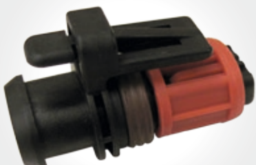
TRU-LOC® Tru-Loc is a 2-pin connector with 1.5 mm socket contacts featuring Amphenol's exclusive RAD-SOK® contact system. The Tru-Loc connector series is designed to perform in demanding environments, such as under valve covers on diesel engines and in various under-the-hood interconnect applications.
