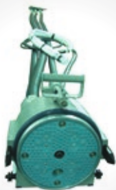
JR JUMPER Inter-car jumper for EMU combine power, signal and fibre system together.
