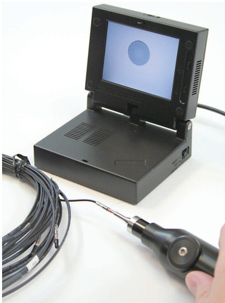
the JDA-1100 Inspecting a Fiber Optic Termini
