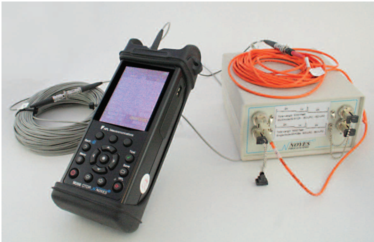
FSP-180 Handheld OTDR Testing a Cable
